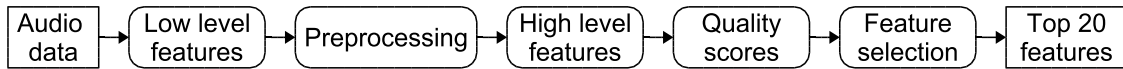
Fig. 1. Processing steps to obtain optimized audio features from raw audio on training data.
